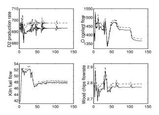
Fig. 4. Pulp mill closed-loop responses: solid line (coordinated); dash line (decentralized)
