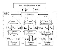
Fig. 3. coordinated, decentralized MPC target calculation  $\label{eq:matrix}$
