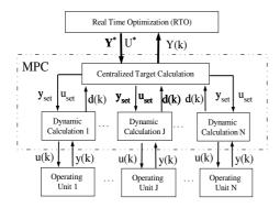
Fig. 2. Centralized MPC target calculation
