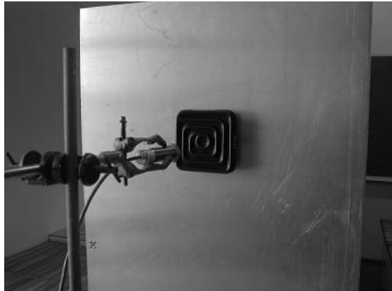
Fig 4. Laboratory arrangement of IR emitter and temperature sensor
