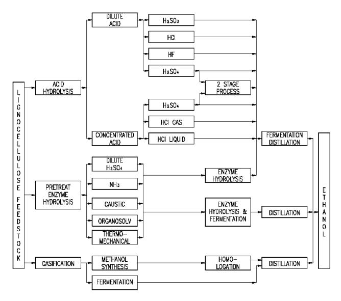
Figure 1. Ethanoi from lignocellulose process matrix.
