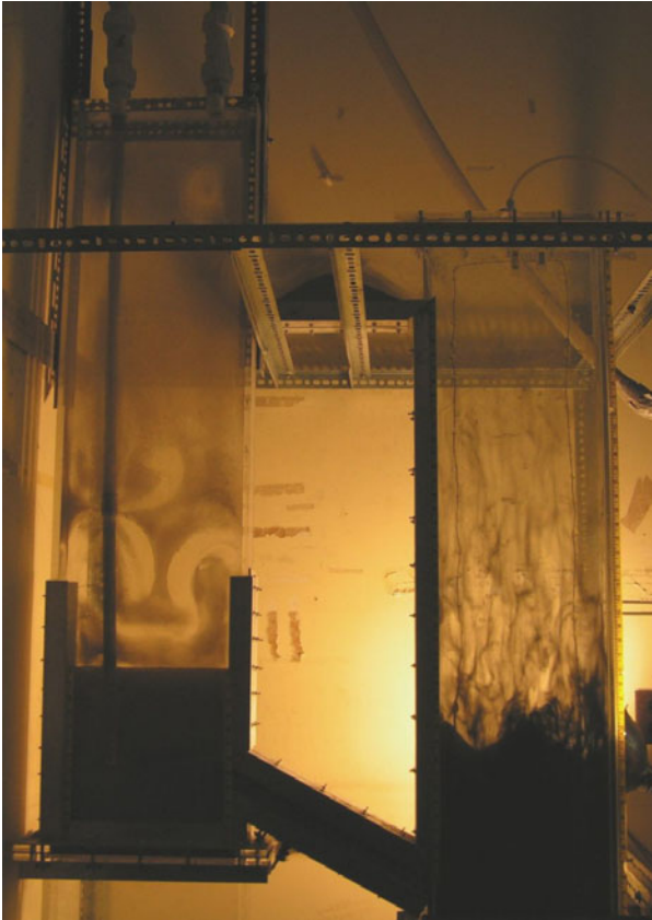
Figure 1: Circulating fluidized bed showing clusters formed by 75 \mu\text{m} FCC particles
