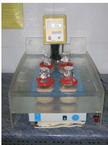
Figure 1. Experimental set-up used for the extraction of \beta -glucans from barley
