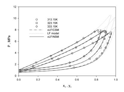
FIGURE 3. Vapor-liquid equilibria (Ref. 32) of the  $CO_2$ /propane system with predictions of the xLF/NSM (solid curves) and the LF EOS(dotted curves).
