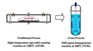
Fig. 7. Reaction Mode Innovation in the Green Process with SMS Media
