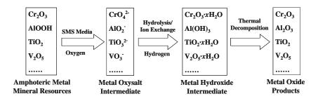
Fig. 10. Target Element Conversion Process for the SMS Platform
