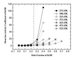
Fig. 3. Relationship of Mean Ion Activity Coefficient and Mole Fraction for Aqueous KOH Solution under Different Temperatures (Data from Li, 1996)
