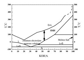
Fig. 1. SMS Region of Aqueous Electrolyte Solution
