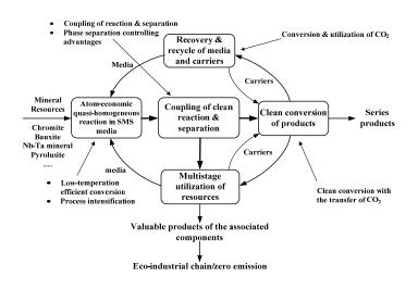
Fig. 11. Technical Route for the SMS Platform (Zhang, 2004)
