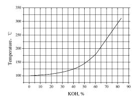
Fig. 2. Relationship of Boiling Point and Concentration for Aqueous KOH Solution
