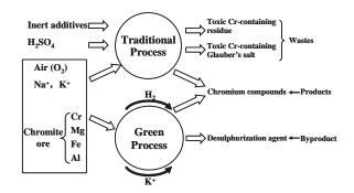
Fig. 6. Raw Materials Substitution in the Green Process with SMS Media
