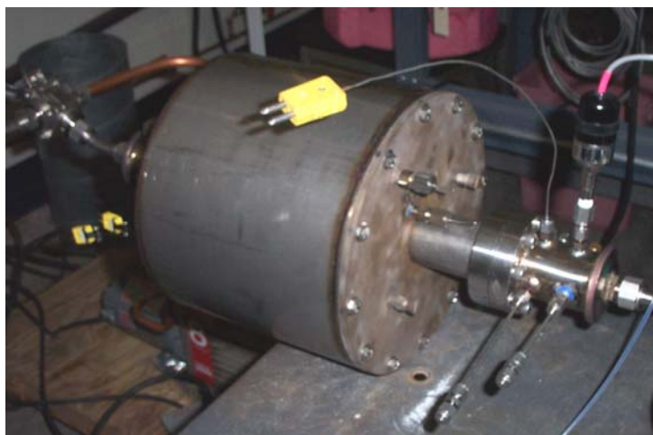
Figure 6. Microlith ® -based regenerable adsorber unit rated for 5-cfm flow rate after integration with the external housing.
