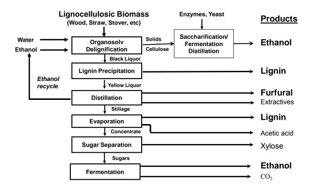
**Figure 1. The Lignol Biorefinery Process**
