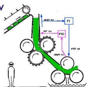
There are integrators in P(z) between speed and chute height and between flap and chute height
