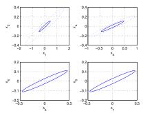
Fig. 2. Visualization of Observability Grammian Ellipsoids
