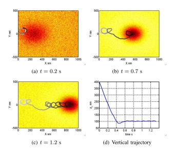
Fig. 5. Tracking a moving particle with velocity  $V=0.62~\mu m/s$ . (a-c) Snapshots of the planar trajectory of the tip. Colors correspond to time with the most recent points in black. (d) The vertical separation of the particle's center and the tip as function of time for a moving particle.
