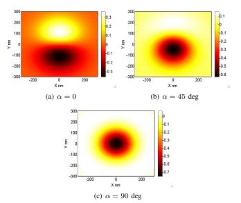
Fig. 2. The phase shift (degrees) for three different values of  $\alpha$ . The tip-sample separation was set to  $z_0=50$  nm and the model parameters to:  $Q=180,\ k=1$  N/m,  $m_z=5.1\times 10^{-15}$  Am²,  $d_m=300$  nm,  $M=480\times 10^3$  A/m (the saturation magnetization of magnetite -  $Fe_20_3$ ) and a=25 nm. The values for  $m_z$  and  $d_m$  are from experiments in [20].
