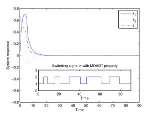
Fig. 2. System response of the closed-loop system in MDADT switching
