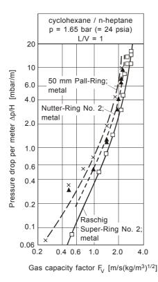
*Fig. 5: Comparison of pressure drop for Raschig Super-Ring No. 2, 50 mm Pall-Ring and Nutter-Ring No. 2. Tests had been performed at FRI facility in StillwaterOklahoma/USA.*
