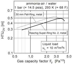
*Fig. 4: Height of an overall gas side mass transfer unit for various gas capacity factors and constant liquid load for 50 mm Pall-Ring and Raschig Super-Ring No. 2 in metal. Tests had been performed at Ruhr University Bochum/Germany.*
