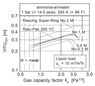
Fig. 8: Comparison of the height of overall gasside mass transfer unit between various sizes of Raschig Super-Rings and the structured packing Ralu-Pak 250 YC for the absorption system ammonia-air/water. Tests had been performed at Ruhr University Bochum/Germany.
