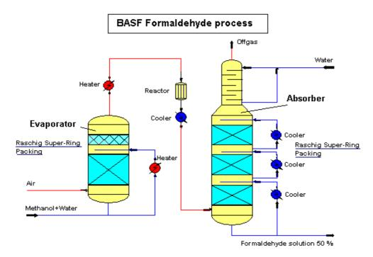
Fig. 14: BASF formaldehyde process with Raschig Super-Rings for production of 50% formaldehyde solution
