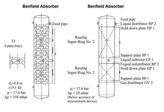
*Fig. 13a: Benfield absorber with 4-path trays before revamp*
