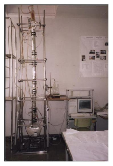
Figure 2. Batch distillation pilot plant.
