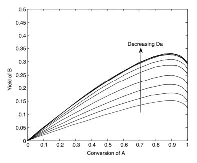
Figure 2. Effect of Damköhler number for reactive condenser model
