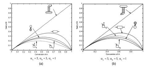
Figure 8. Feasible regions with different relative volatilities for reaction system  $A \rightarrow B \rightarrow C$
