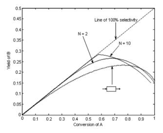
**Figure 11.** Yield *vs* conversion plot for maximum boiling azeotrope b/w A-B for reaction system  $2A \rightarrow B$ ,  $A + B \rightarrow C$ : N is the number of stages required in the *reactive rectification* unit
