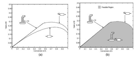
**Figure 13.** Yield vs conversion plot for maximum boiling azeotrope b/w A-B for reaction system  $2A \rightarrow B$ ,  $A + B \rightarrow C$ : N is the number of stages required in the *reactive rectification* unit
