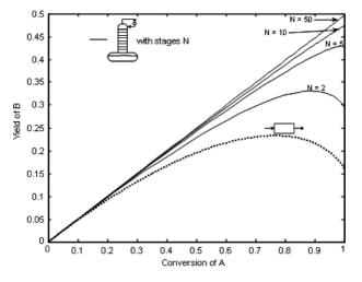
Figure 5. Effect of number of stages (N) on feasible region of reactive rectification unit
