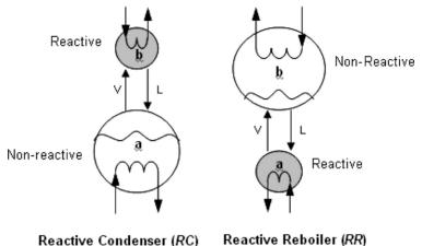
Figure 1. Reactive condenser and reactive re-boiler models
