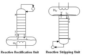
Figure 3. Reactive rectification and reactive stripping models
