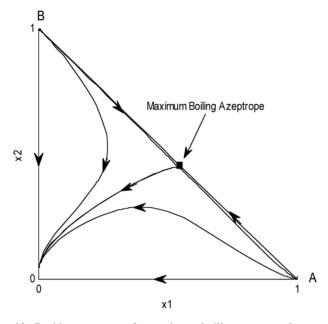
Figure 10. Residue curve map for maximum boiling azeotrope between A-B
