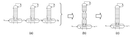
Figure 4. Continuous reactive rectification models
