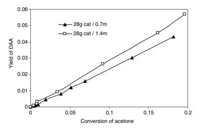
Figure 7. Yield vs conversion at 28g catalyst loading and 0.6KW re-boiler duty
