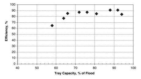
Figure 3. Efficiency of ULTRA-FRAC trays in depropanizer service
