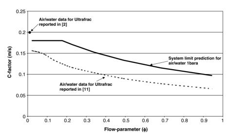
Figure 5. Maximum (air/water) capacity data for ULTRA-FRAC taken from references [2,11]
