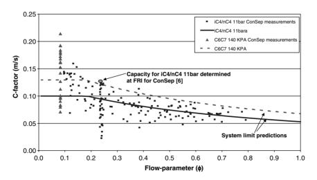
**Figure 4.** ConSep hydrocarbon data (iC4/nC4 11bar circulation and total reflux runs + C6C7 140 KPA total reflux runs)
