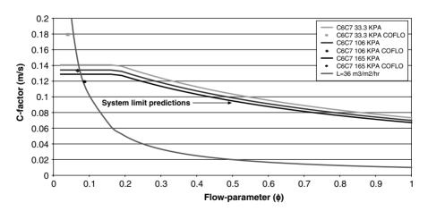
Figure 1. COFLO [9] flood points at different pressures compared with the system limit correlation
