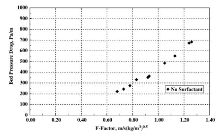
Figure 3. Measured bed pressure drop (without surfactant)
