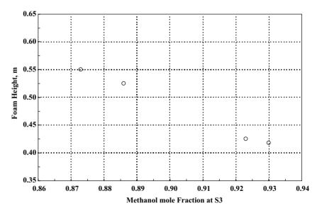
Figure 5. Effect of methanol concentration on foam height
