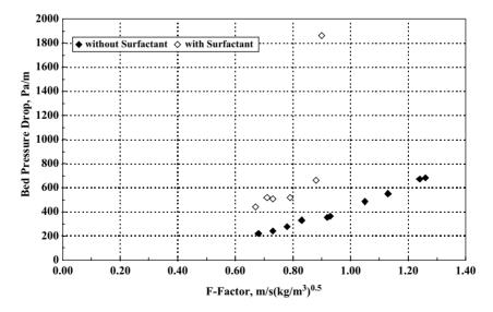
Figure 7. Effect of foaming on bed pressure drop
