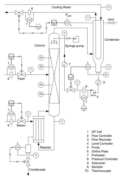
Figure 1. Schematic diagram of experimental setup
