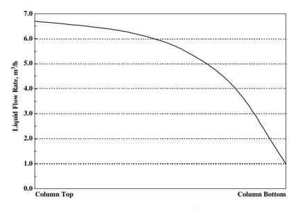
Figure 4. Volumetric flow-rate profile of a methanol/water distillation column
