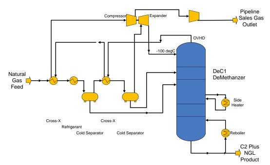
Figure 1. Process Flow Diagram for Simple GSP Plant
