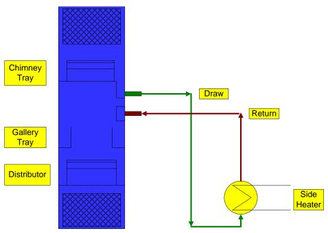
Figure 2. Typical Side Heater Arrangement
