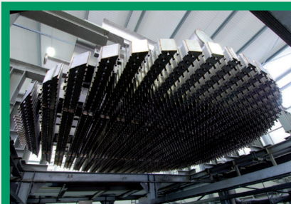
Raschig test stand - 12 m diameter and liquid loading to 2400 m 3 /h
