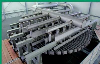
Raschig test stand - 12 m diameter and liquid loading to 2400 m 3 /h
