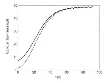
Fig. 4. Simulation results : the biomass concentration X and its on-line estimate  $\hat{X}$  (dotted line)
