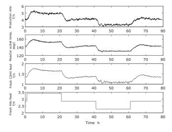
Fig. 5. Simulation results for  $\pm 20\%$  step changes in the fresh HAc feed rate.
