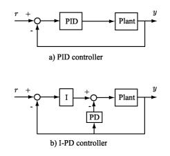
Fig. 2. Two different implementations of PID controller. a) standard PID controller, b) I-PD controller.
