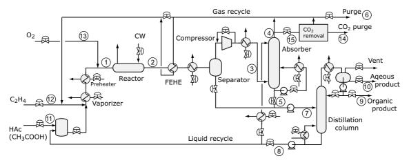
Fig. 1. Process flow diagram of the vinyl acetate monomer production plant. The stream numbers are the same as those of the original paper (Luyben and Tyreus, 1998).
