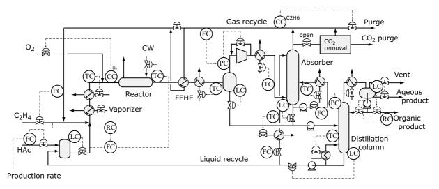
Fig. 4. An alternative control loop configuration. The fresh acetic acid feed is on flow control to set the production rate. A cascade loop from the liquid reactor feed flow to the reactor temperature setpoint is incorporated to ensure regulation of the acetic acid inventory.
