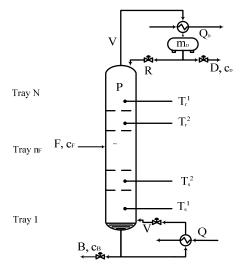
Figure 1. Schematic of a distillation column
