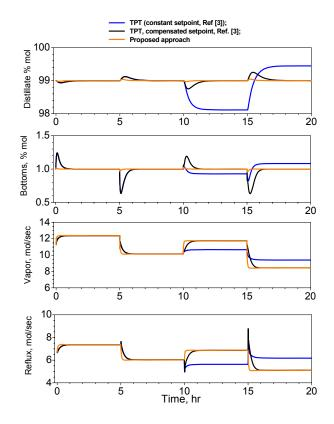
Fig. 2. Closed-loop response of the column to a sequence of feed flow rate and composition disturbances.
