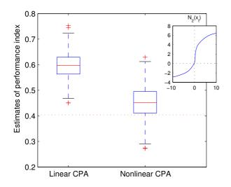
Fig. 4. Comparative box plots of the quality estimates of the performance index for a Wiener model. The horizontal dotted line is the true value of 0.404.
