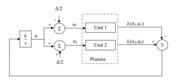
Fig. 1. Schematic for multi-unit optimization
