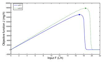
Fig. 3. Static characteristics of the two non identical bioreactors
