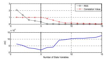
Fig. 1 Plot of RSS, correlation values diagonal of S matrix, and AIC. State variable selection is 5.
