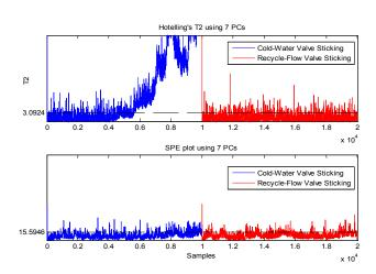
Fig. 4 Detection of Cool-Water and Recycle flow valve sticking using  $T^2$  and Q statistics of a PCA model.
