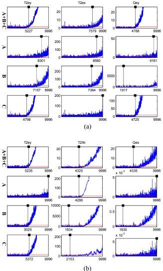
Fig. 3. (a)  $T^2$  on output and state residual, and Q statistics on the output residuals for heat exchanger fouling fault (b)  $T^2$  statistics on output residual and state vectors, and Q statistics on state residuals for temperature sensor drift fault.
