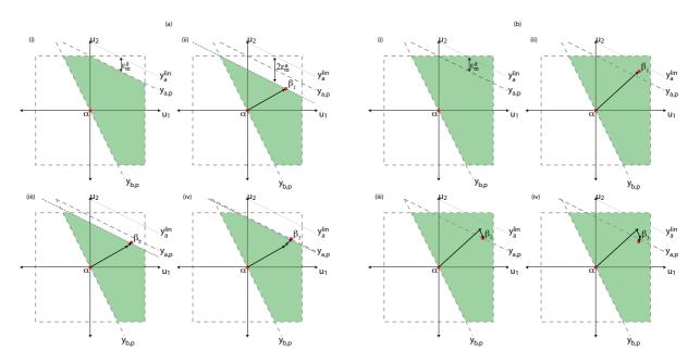
Fig. 4. Theoretical illustration of the HCC (a) and SCC (b) approaches for a problem that involves going from a steady-state operating point  $\alpha$  to a new steady-state operating point. The FR is shaded.
