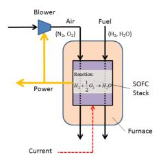
Fig. 1. Diagram of the SOFC stack system.
