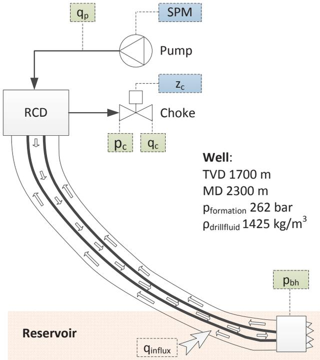
Fig. 1. Illustration of the well.
