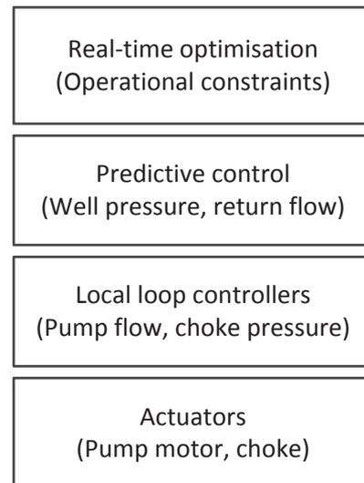
Fig. 2. Illustration of the different control levels.
