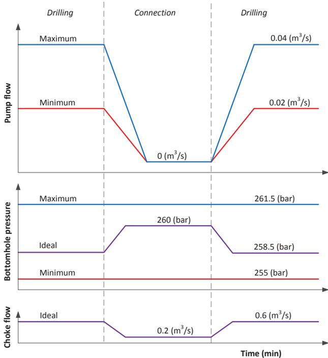
Fig. 3. Connection procedure.
