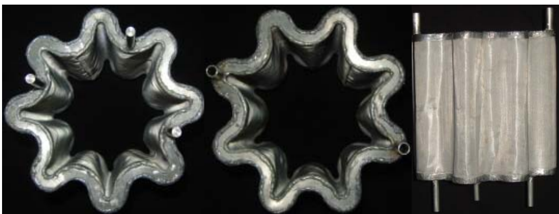
Fig. 1 Upper (a) and lower (b) cross view and axial view (c) of the design filtration module.
