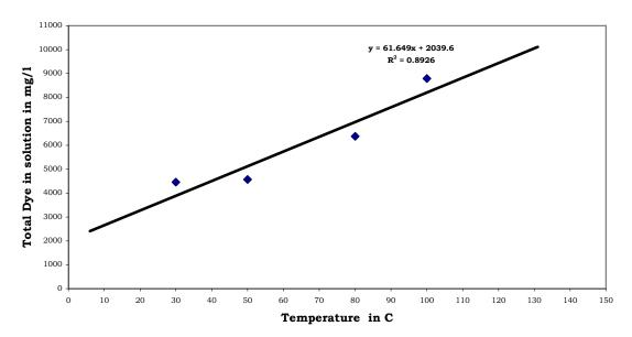
Figure1: Temperature effect on extraction of dye from Marigold flower
