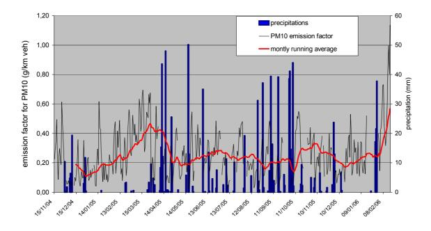
Figure 4: Calculated PM<sub>10</sub> emission factor (exhaust + non-exhaust) in Cuneo
