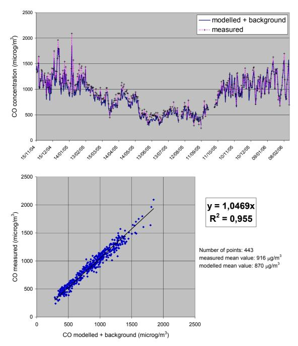
Figure 6: Comparison of measured and modelled CO daily mean concentrations in Cuneo
