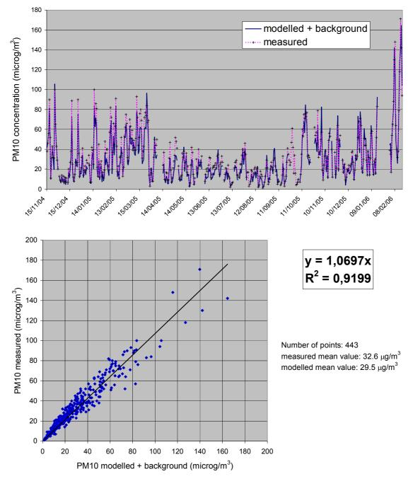
Figure 7: Comparison of measured and modelled PM<sub>10</sub> daily mean concentrations in Cuneo
