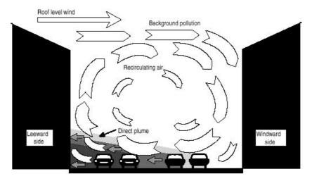
Figure 5: Conceptual scheme of the OSPM model
