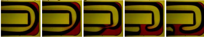
(b) New liquid plug forming at the second bend ( V_{sw} = 0.002 m/s, V_{sa} = 0.75 m/s)
