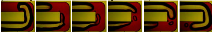
Figure 7. Flow pattern observed at two 90 degree bends at 1 mm from each other.
