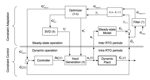
Figure 1. Scheme combining constraint adaptation and constraint control.
