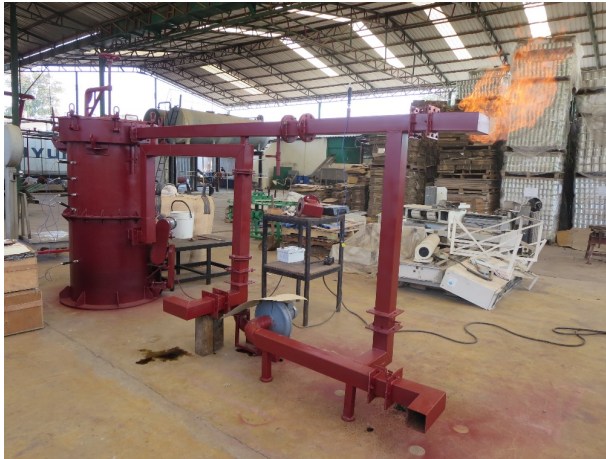
Figure 2 The experimental setup of the downdraft gasifier
