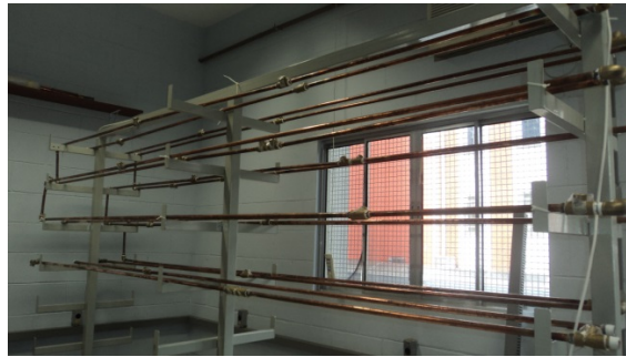
Figure 1. Experimental leak detection system in gas piping.
