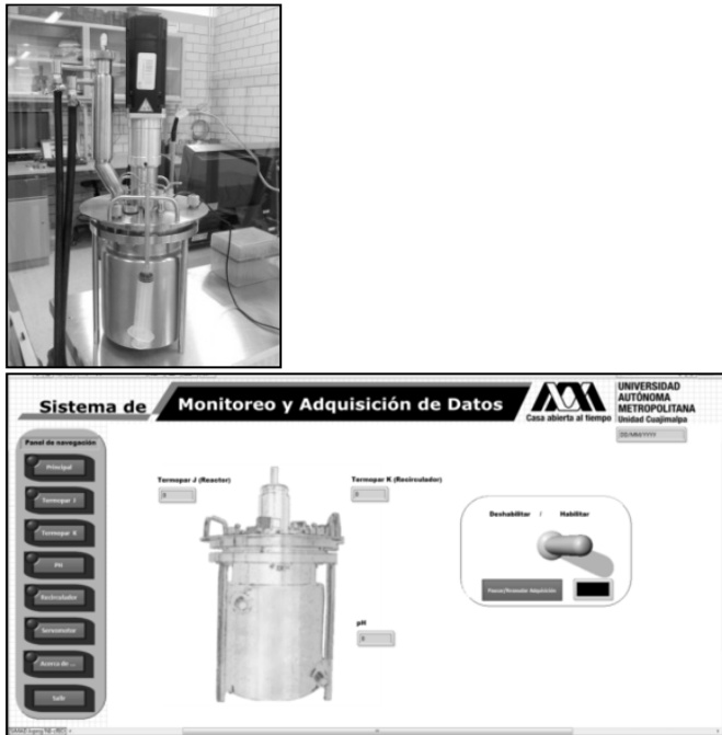
Figure 1. Experimental system: (a) reactor and (b) data acquisition and control system.
