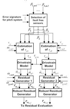
Fig. 3. Diagnostic scheme for drivetrain subsystem.
