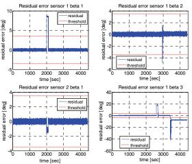
Fig. 5. Residual for sensors  $r_{\beta_1}$  and  $r_{\beta_2}$  of pitch subsystem 1 and sensor 1 ( $r_{\beta_1}$ ) of pitch subsystems 2 and 3.
