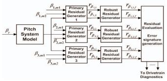
Fig 2. Diagnostic scheme for the three pitch subsystems.
