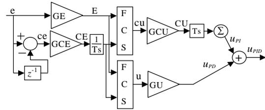
Fig. 1. PI-FLC + PD-FLC structure for a PPID-FLC.
