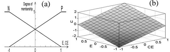
Fig. 4. (a) Membership functions for E and CE; (b) Control surface of the normalised and linear FCS.
