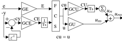
Fig. 3. Modified HPID-FLC structure.
