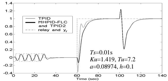
Fig. 9. Comparison of set-point and load disturbance responses for  $G_4(s)$ .
