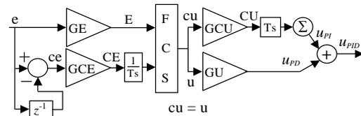
Fig. 2. Structure for an HPID-FLC.
