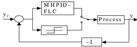
Fig. 5 Relay feedback experiment.
