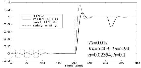
Fig. 7. Comparison of set-point and load disturbance responses for  $G_2(s)$ .
