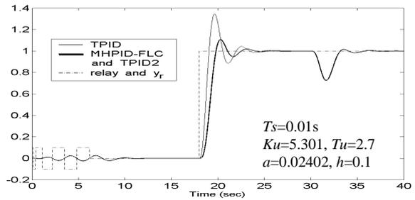
Fig. 8. Comparison of set-point and load disturbance responses for  $G_3(s)$ .
