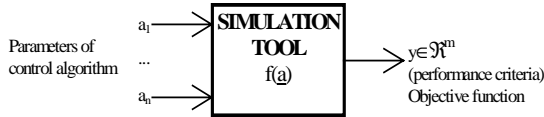
Figure 2: The role of the simulation tool as a means to evaluate the objective function
