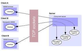
Figure 3. Remote simulation environment with concurrent clients
