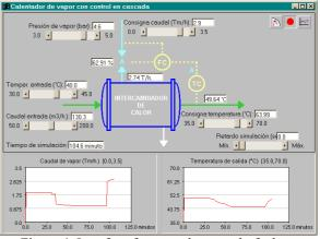
Figure 4. Interface for cascade control of a heat exchanger
