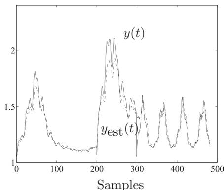
Fig. 3. Comparisons between the process and the estimated model outputs with identification data.
