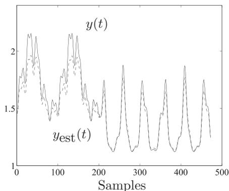
Fig. 4. Comparisons between the process and the estimated model outputs with validation data.
