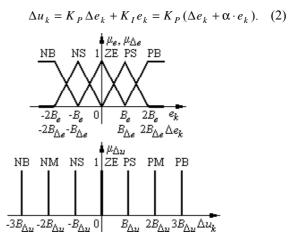
Fig. 3. Membership functions of input and output linguistic variables in B-FC.
