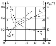
Fig. 5. Control system performance indices versus  $\beta$ .
