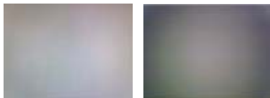
(a) Good Auto-Iris image (b) Auto-Iris defect image Fig. 17. Auto-Iris inspection
