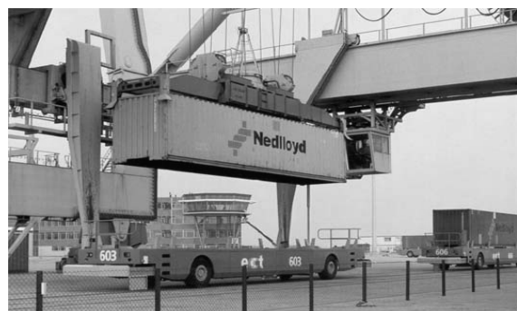
Fig. 1. An AGV operating in the ECT at Port of Rotterdam, the Netherlands.
