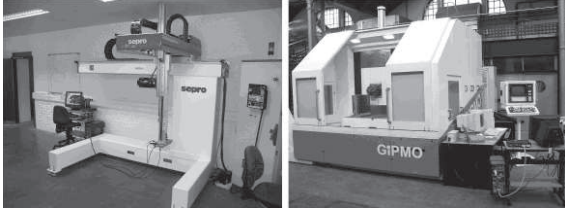
Fig. 1. Left: 3-axis Cartesian robot (max feedrate: 120 \text{ m}\cdot\text{min}^{-1} , max acceleration: 4 \text{ m}\cdot\text{s}^{-2} ); Right: High dynamic machine-tool prototype (max feedrate: 100 \text{ m}\cdot\text{min}^{-1} , max acceleration: 20 \text{ m}\cdot\text{s}^{-2} , actuators: permanent magnet linear synchronous motors).
