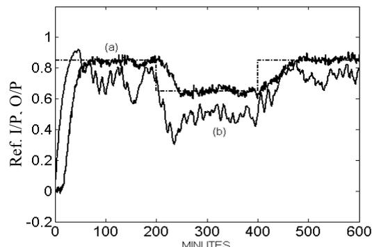
Fig. 9 Performance of the extended SOFLC algorithm including a 3<sup>rd</sup>-order filter; (a): output signal ; (b) input signal
