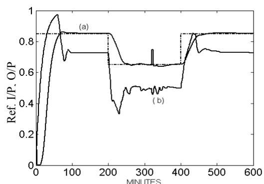
Fig. 7 Closed-loop control simulation results with added noise; (a): output ; (b) input
