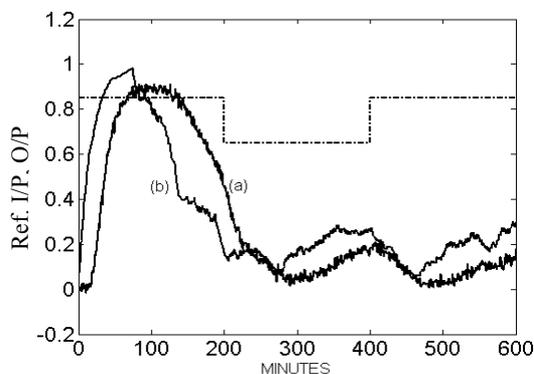
Fig. 8 Closed-loop control simulation results when noise is added to the output; (a): output signal ; (b) input signal
