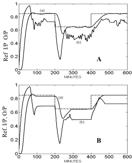
Fig. 4 Closed-loop control simulation results using the new SOFLC algorithm (A); and the standard SOFLC algorithm (B) (a): output signal ; (b) input signal
