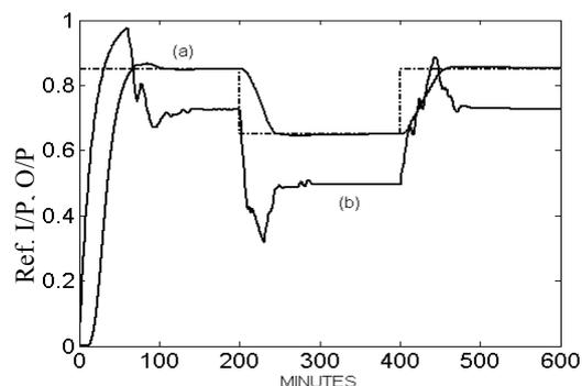
Fig. 6 Closed-loop control simulation results using the new improved SOFLC algorithm; (a): output signal ; (b) input signal
