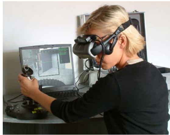
Fig. 5. Orpheus operator's station for telepresence control
