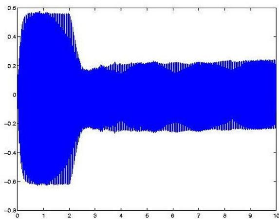
Fig. 7. Imperfect rejection due to frequency mismatch
