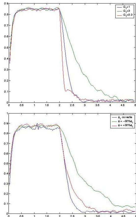
Fig. 8. Comparison of envelopes/time (top: gain mismatch, bottom: phase mismatch)
