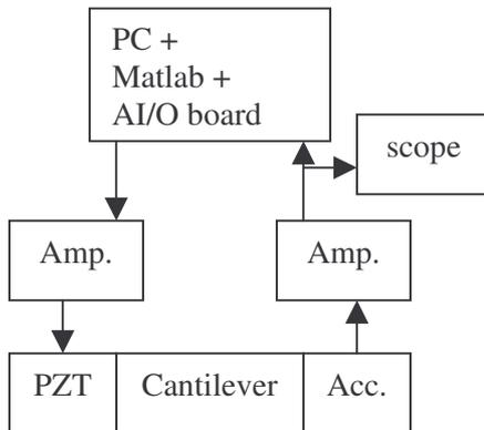
Fig. 2. Experimental set-up (principle)
