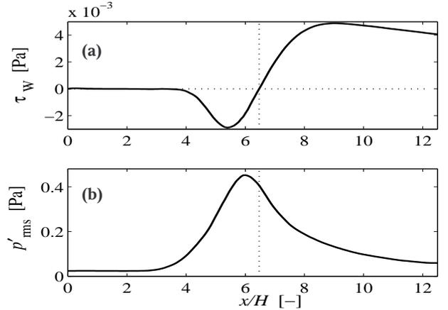
**Fig. 2.** Wall-shear stress (a) and wall pressure fluctuations (root-mean-square value) in the wake of the step. The  $x$ -direction is normalised by the step height  $H$ .
