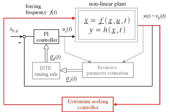
**Fig. 5.** Scheme of the proposed closed-loop.
