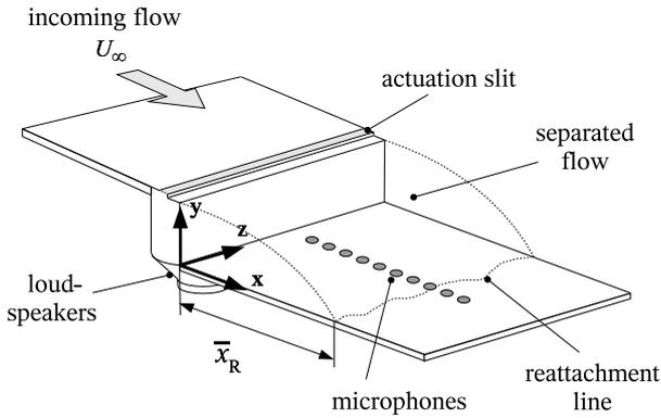
**Fig. 1.** Flow configuration: The backward-facing step with loudspeakers used for actuation.
