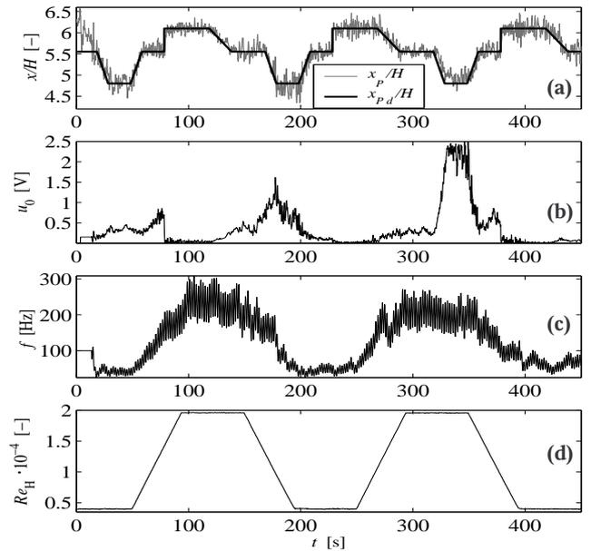
**Fig. 7.** Closed-loop control of the reattachment length behind a backward-facing step at variable Reynolds numbers (wind tunnel experiment).
