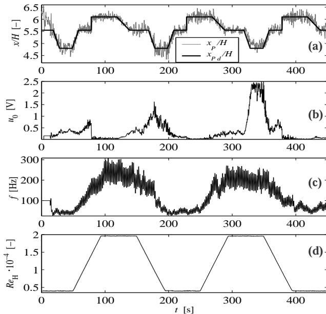
Fig. 10. Closed-loop control of the surrogate variable describing the reattachment length for variable Reynolds numbers.
