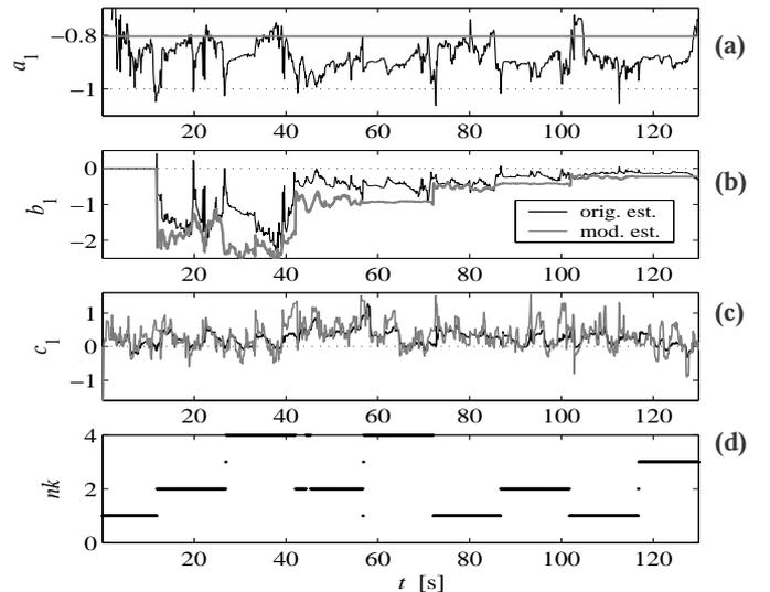
**Fig. 9.** Estimated parameters of an ARMAX model at a Reynolds number  $Re_H=4000$  exploiting an approximation of the non-linear sensor dynamics.
