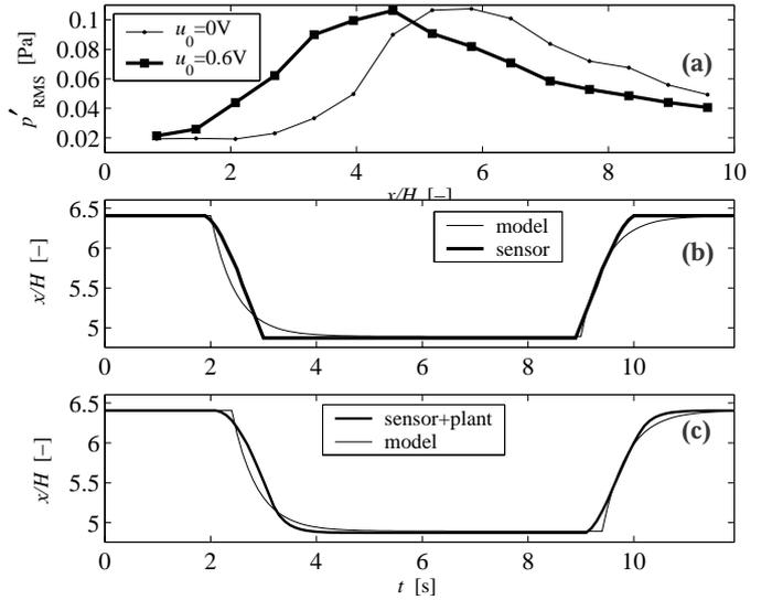
**Fig. 8.** RMS value distribution for a natural and a manipulated flow (a) and the response of an estimated model describing the non-linear sensor dynamics (b), (c).
