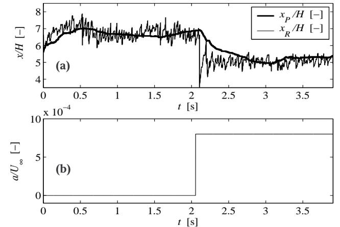
**Fig. 3.** Step response of the instantaneous reattachment length  $x_R/H$  and the surrogate length  $x_p/H$  based on the wall-pressure fluctuations behind a backward-facing step. Large-Eddy-Simulation (LES) at  $Re_H = 4000$ .
