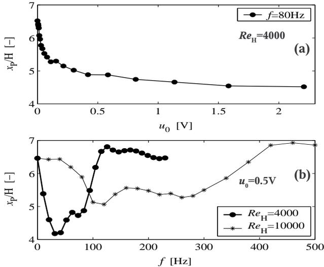
**Fig. 4.** The surrogate variable as a function of the forcing amplitude (a) and the forcing frequency of the control signal, see eq. (1), for different Reynolds numbers (b).
