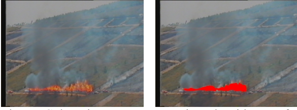
Fig. 5. Colour images segmentation algorithm. Left, original image. Right, detected fire.
