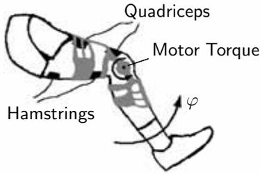
Fig. 1. Motor-driven orthosis and electrically stimulated muscles (quadriceps and hamstrings) to control the knee bend angle  $\varphi$ .
