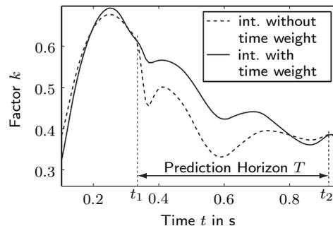
Fig. 6. With time weighted integration, the factor  $k$  adapts more gradually to an upcoming instantaneous frequency change of the reference signal  $w$  (at  $t_2$ ), which is predicted at  $t_1$ .
