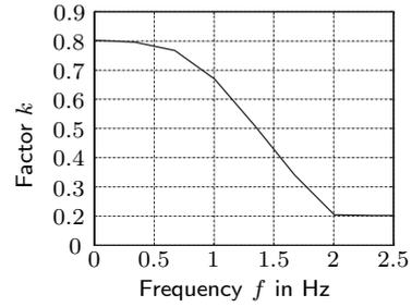
Fig. 5. The parameter  $k$  as a function of the frequency  $f$  of a sinusoidal reference signal. Both actuators always participate with a minimum portion of 20%.
