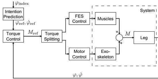
Fig. 3. Based on the predicted reference angle trajectory, the model-based torque controller predicts an optimal torque trajectory, which thereafter is split up to the two actuators.
