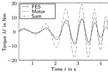
Fig. 7. Torque distribution: The motor portion increases with the frequency of the reference torque, the muscle portion decreases.
