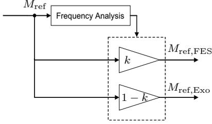
Fig. 4. The reference torque is split up to the FES-stimulated muscles and the motor-actuated exoskeleton via an adaptive, frequency-dependent convex combination.
